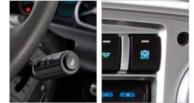
Engine brake and Intarder operating lever: You can manually activate the auxiliary brakes, or you can enable the vehicle to set it automatically for you.
