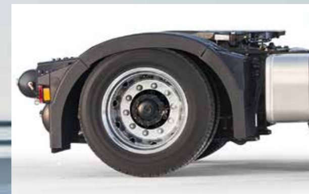
Low Liner: You can also choose the Low Liner version with a 5 th wheel height that can be lowered down to 980 mm as preferred.
