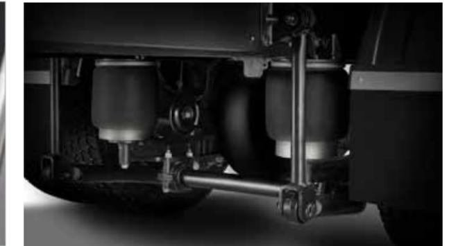
The newly developed rear air suspension is developed for the 4x2 and 6x2 models. In addition to the unique driving comfort, it guarantees much safer transport of fragile loads.
