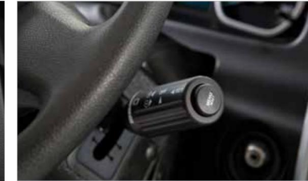
The 600 KW Intarder, which is available as an optional feature on vehicles, meets all expectations under such challenging conditions as going downhill while loaded. Preventing unnecessary use of your service brake, it prolongs service life.
