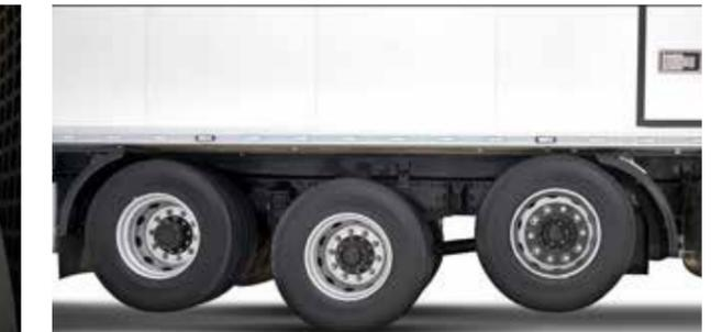
For vehicles with 6x2 and 8x2 axle type, in unloaded conditions, the rear axle is off the ground. This mechanism avoids unnecessary tire wear. When the vehicle is stopped for loading, tires automatically drop down, thanks to the Auto-drop feature.
